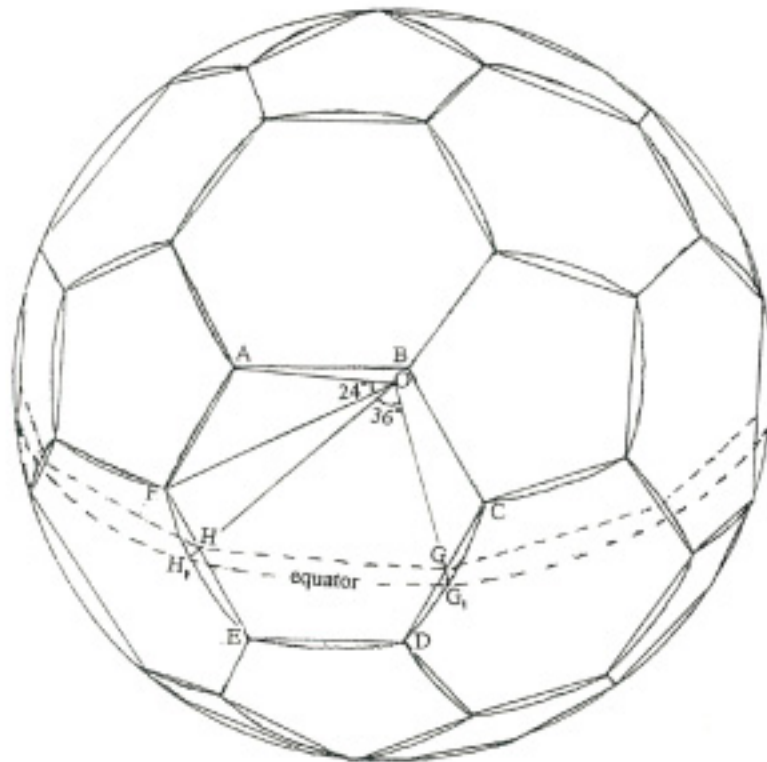
A composite diagram of the hexpenhedron insphered within the football (Note that the sides of the sphero-geometric hexagons and pentagons on the football are curved, and the sides of the hexpenhedron insphered within are straight)
